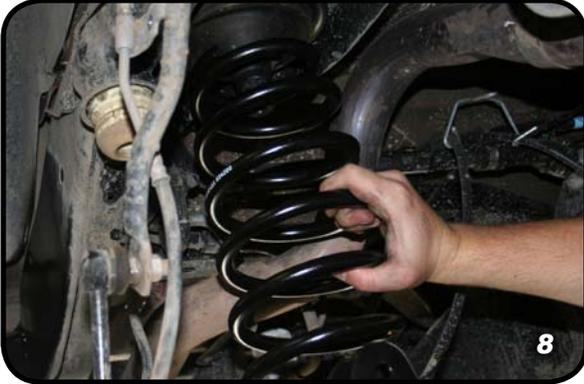
11. Install the new rear springs. Make sure to reuse the factory spring isolator.
