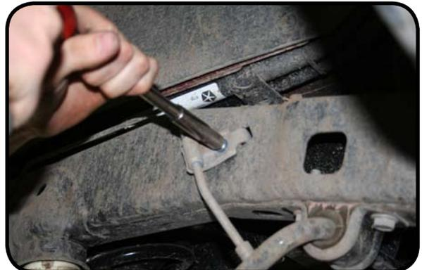
10. Carefully lower the rear axle far enough to remove the rear springs. Be careful not to let the coils fall out as you lower the axle. You will want to lower the axle far enough to install the new 1.5" springs in place. While lowering the axle make sure the brake lines, ABS wires and axle vent do not stretch as this could cause damage to these vital parts.
