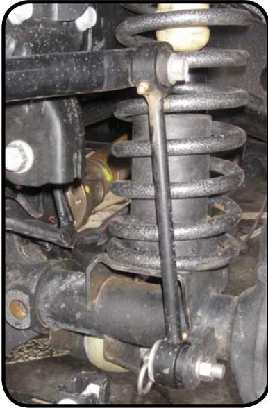
22. Reinstall the lower shock bolts and torque to 56 ft-lbs.
