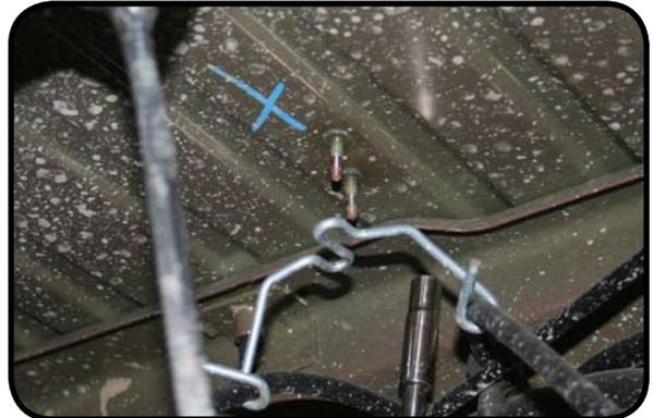
9. Remove the brake line mount at the frame using a 10mm socket.
