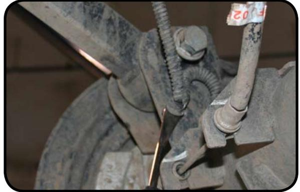
8. Remove the bracket that holds the park brake cables to the body using a 10mm deep well socket.
