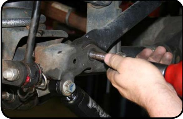
2. Loosen all control arm bolts using a 21mm socket, DO NOT REMOVE ARMS OR BOLTS!
