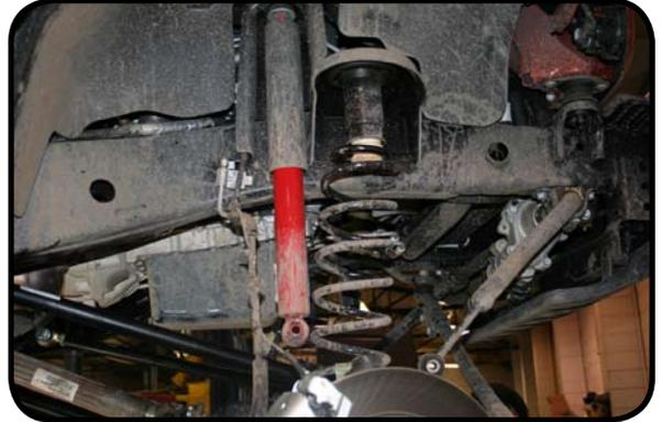
18. Remove sway bar links using 18mm socket and wrench at the axle and 18mm socket and 20mm wrench at the sway bar. Lower the jack enough to remove the springs.
