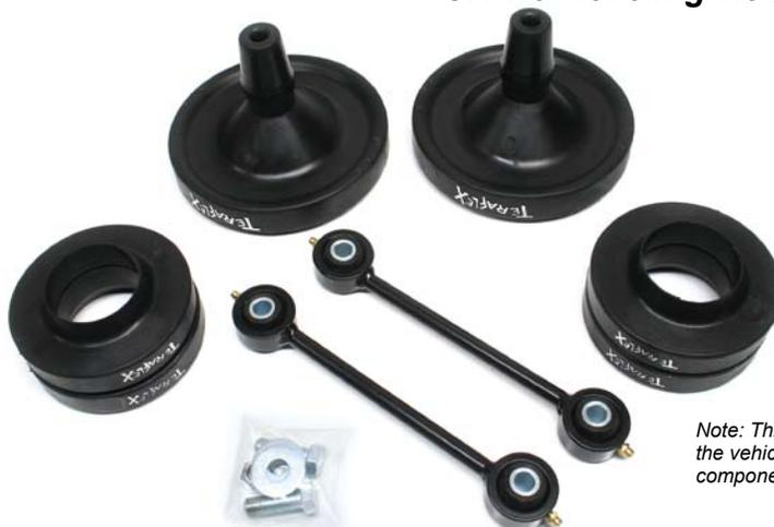
Note: This kit will lift the front of the vehicle 2" and the rear 1" if all components are used.
