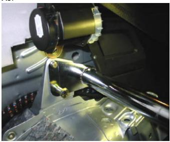
After Test fitment, remove bolts and Reinstall Belt Reels; to do so unwind the belts from the housing first, then you will see the hole at the top of the seat belt housing.
