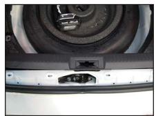
STEP 3 Carefully unclip and remove the trunk sill panel.
