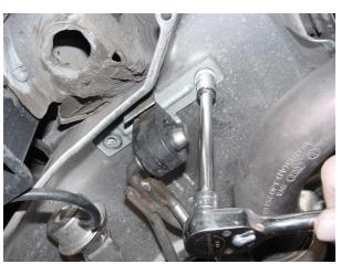
3. Loosen exhaust clamp (17mm Hex) and disconnect exhaust from catalyst. Disconnect left and right exhaust hangars and vacuum hose from diaphragm.
