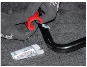
8. Apply supplied grease to inside of supplied bushing and install bushing onto supplied bar. (Left side shown, repeat for right side)
