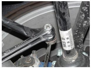
6. Disconnect end links from anti-roll bar by securing stud with 17mm wrench and loosening nut with 16mm wrench. (Left side shown, repeat for right side)
