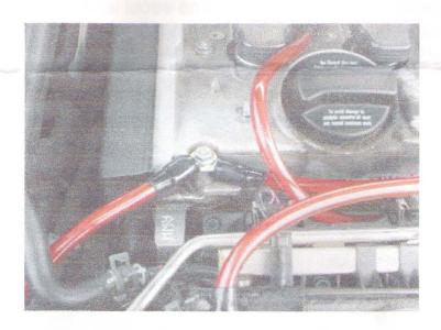
12. Now take the last remaining wire connected to the bracket – and run it around to the throttle body – there is a small bracket that sits next to it...it also holds the engine cover – take out the 10mm bolt (you may need to disconnect the sensor on top of the throttle body to get a clear shot at the bolt – DO NOT FORGET TO RE-CONNECT – you WILL get a check engine light if you don't)...The picture on the next page shows how it should look – you can run the wire under the sensor wire
