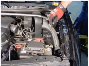
3. Remove side air duct by removing one (1) 10mm hex nut.
