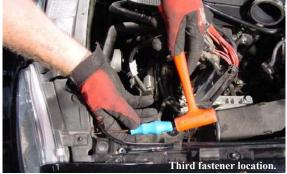
7. Remove the lower air duct housing by removing three (3) push fasteners. To release fastener, punch out center pin with a long reach screwdriver and mallet. NOTE: First push fastener is located between driver's side headlight and grill. Second push fastener must be released from underneath the vehicle. Third fastener is located directly behind the driver's side low beam.
