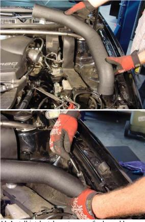
11. Install intake tube onto upper fender and lower isolator mount using washer and nyloc nut (10mm).
