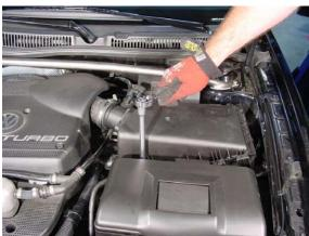
1. Remove entire factory air box by disconnecting Mass Airflow meter (MAF) electrical connector, air pump connection, intake tube, and two (2) 10mm hex mounting bolts.
