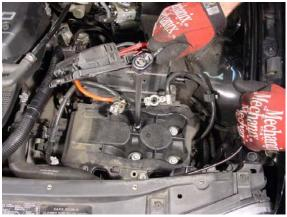
6. Remove two (2) 10mm hex bolts securing fuse block to battery tray. Remove lower battery tray by removing four (4) 10mm hex bolts.
