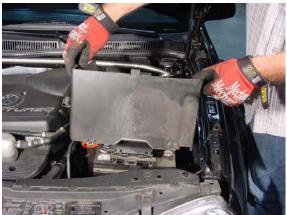
2. Remove battery box by removing one (1) 10mm hex bolt. Pull straight up to remove.
