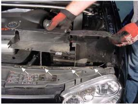
4. Remove four (4) Phillips screws securing upper air duct to core support.
