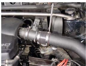
13. Install MAF to factory intake hose and tighten clamp. Install reducer hose and clamps onto MAF and intake tube. Tighten remaining hose clamps.
