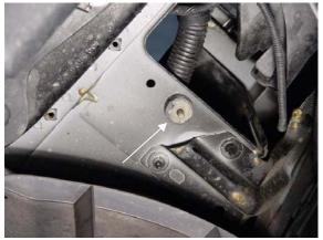
10. Install rubber isolator into existing hole from underneath the vehicle using supplied washer and M6 nyloc nut.
