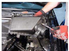
9. Remove MAF from air box lid by removing two (2) Phillips screws.
