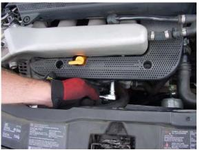
14. Attach air pump tube to fitting by loosening clamp at the engine and extending hose to intake tube fitting.
