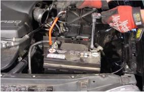
5. Disconnect and remove battery from vehicle.
