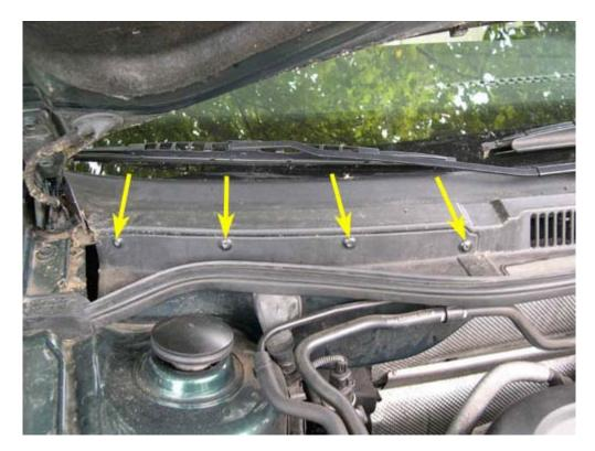
3. Pull up on the rear hood seal (yellow arrow in picture below) and move it out of the way. Begin to remove the pollen filter plenum cover by lifting the front edge slightly to clear the lip at the front of the plenum (metal) and then pulling toward the front of the car (red arrows).
