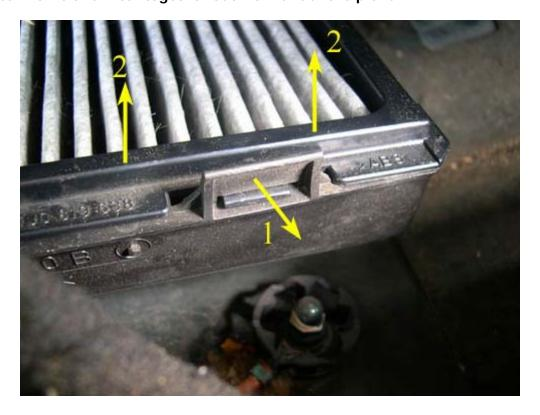
7. The picture below gives a better view of how much pollen and debris the filter actually prevents from getting into the cabin of the car. While the filter in the picture had not been changed in about 50k miles, I routinely scraped the pollen and debris out from between the fins. The space between the fins was free of pollen and debris only 4k miles before these pictures were taken.
