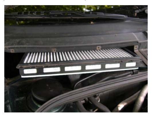
12. The picture below shows the filter frame and filter correctly reinstalled. If the reinstallation is done correctly, the two retaining tabs on the front edge of the frame should click into place easily and there should be no gaps between the filter frame and the top of the blower motor assembly on the sides. It's hard to describe, but you'll be able to tell when the frame and filter are installed correctly.
