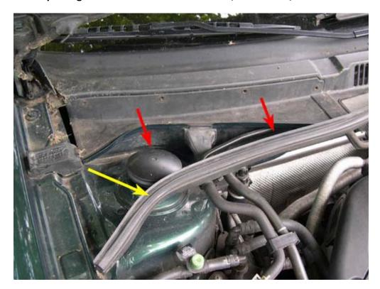
4. After pulling the cover part way out, you'll need to lift it up slightly to allow two wide tabs on the bottom of the cover (indicated by the arrows in the picture below) to clear the lip at the front of the plenum.
