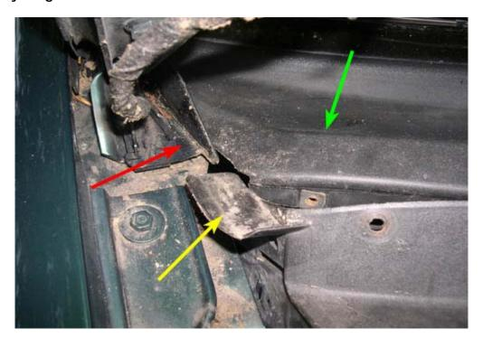
14. One the cover is back in place, put the four T25 Torx screws back in, re-install the rear hood seal and you're done.
