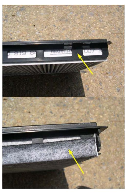
10. On the rear edge of the filter frame, there are three small tabs which must slide into corresponding slots when the filter frame and filter are reinstalled under the plenum. One of these tabs is shown in the picture below.
