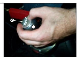
STEP 56. Again, test movement of shifter into all gears. DO NOT operate vehicle until all gears can be smoothly and <u>fully</u> enganged.
