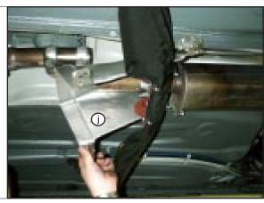
STEP 40. Reinstall heat shield snap washers (e). TOOL: Screwdriver (Flat) (T)
