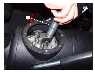
STEP 49. Test movement of B&M Shifter (A) into all gears concentrating on the 1-2 shift and reverse. Adjust Slider (I) assembly and lock by tightening Jam Nut (V).
