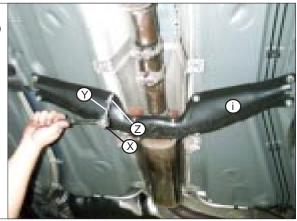
STEP 13. Remove center heat shield (j).
