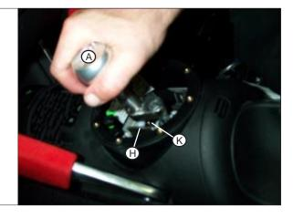
STEP 50. Remove Knob (B). Install collar into rubber boot and then over the **B&M** Shifter (A).
