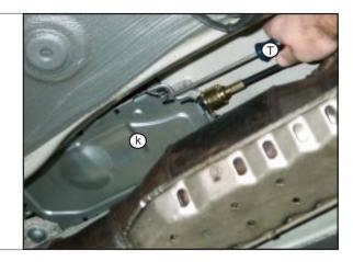
STEP 15. Remove retaining clip m from shifter.
