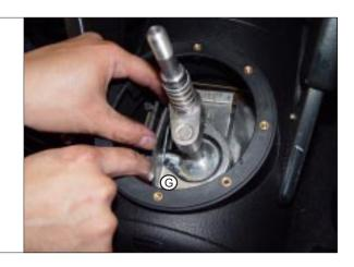
STEP 31. Reinstall two (2) plate screws (f). TOOL: Torx Drive (T-20) (S)
