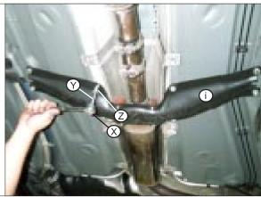
STEP 42. Slide exhaust coupling (g) back over both pipes.
