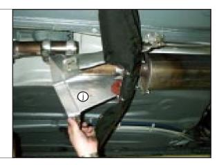
STEP 14. Carefully pry bottom plate (k) off of shifter enclosure.
