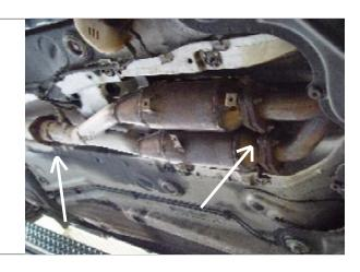
STEP 11. Remove front heat shield (b).
