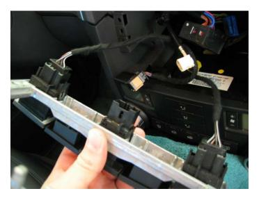
7. Firmly pull vent and storage assembly straight out toward rear of vehicle. The entire assembly will pop out.
