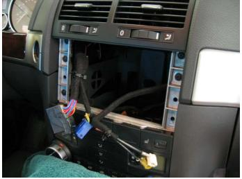
4. Remove 6 torx (T20 size) screws from exposed metal bracket. Three screws will be on each side.
