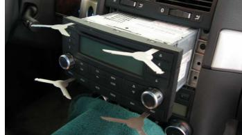
2. Remove 4 radio tools by pulling outward firmly.
