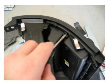
10. Use a longer screwdriver inserted between vents and old storage bin to release 4 tabs and allow old bin to completely release up and out of assembly.
