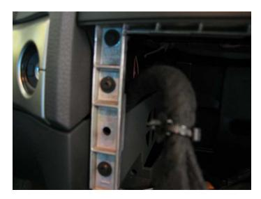
5. Gently pull bottom of bracket out by pulling from behind hazard and seat heater controls. Complete metal bracket will slide out from under vents.
