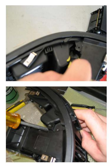
11. Remove old assembly and insert new Dash Storage Bin & Cover. Rear of bin will catch on vents and hold it in place.
