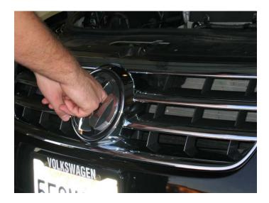
2. Using Torx T25 bit, remove single screw behind hole where emblem was located.
