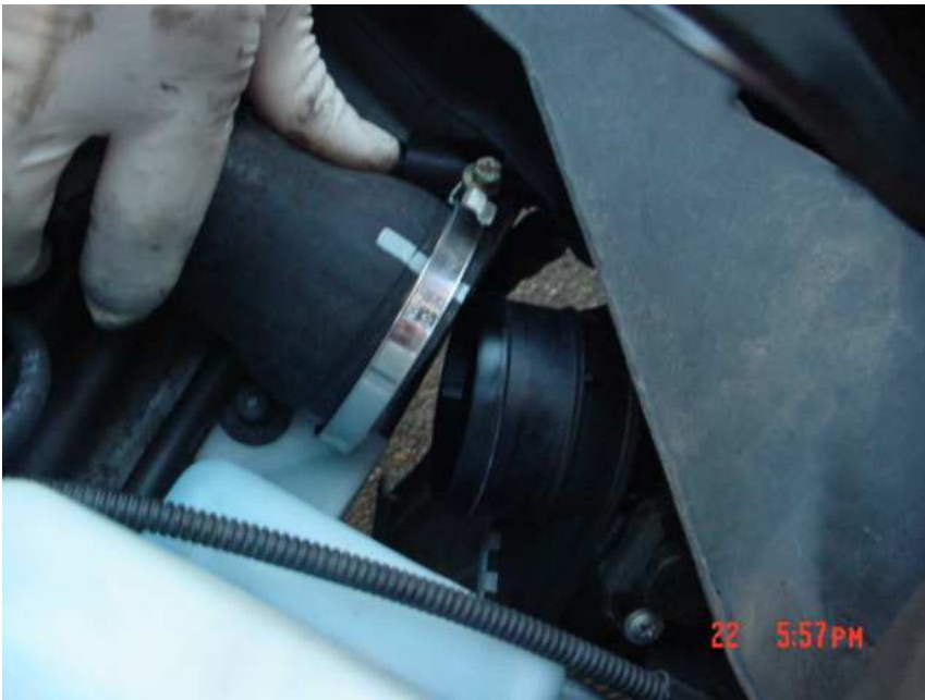
Gently remove the intercooler. Disconnect the MAP Sensor connector(located on top rear side of the stock intercooler)as you pull out the IC:
