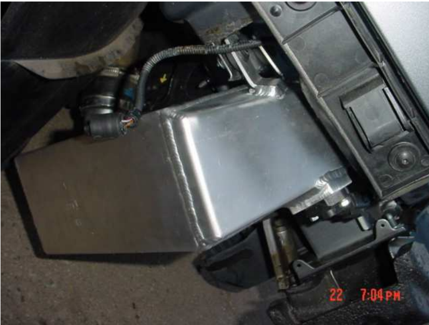
Connect the MAP sensor(which is now on the front of the intercooler):
