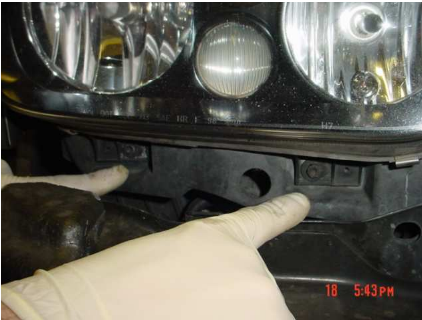
Gently slide the headlight out and disconnect it from the factory wiring harness:
