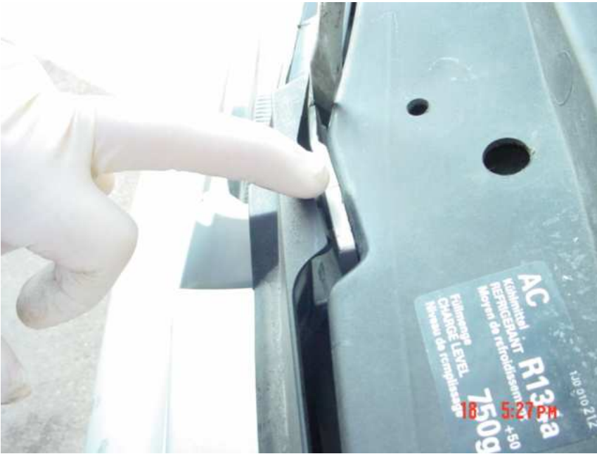
Pull outwards and upwards to release the retaining clips along the bottom edge of the grill:
