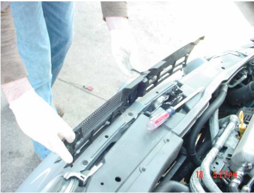
Pull the stock grill off of the vehicle, and place to the side.
