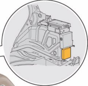
Adaptive suspension control unit J197 on right in luggage compartment
