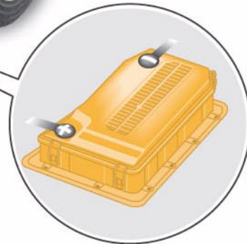
Onboard power supply battery under driver's seat
