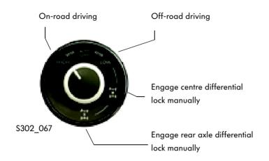
The **"HIGH"** setting is for on-road driving. The differential locks are engaged automatically depending on the situation (e.g. icy conditions). In this case, the differential lock is not closed to 100%, as for example with a constant mesh coupling, but is engaged with a soft setting. The off-road reduction stage is not engaged.
