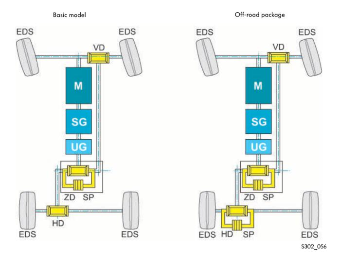
M - motor; MG - manual gearbox; RG - reduction gearbox; CD - centre differential; RD - rear axle differential; FD - front axle differential; DL - differential lock; EDL - 4-wheel brake intervention
