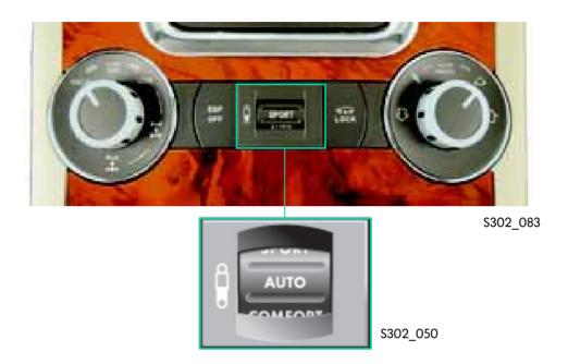
In the Touareg, you set the damping using the damping regulator switch in the middle of the chassis control panel.
