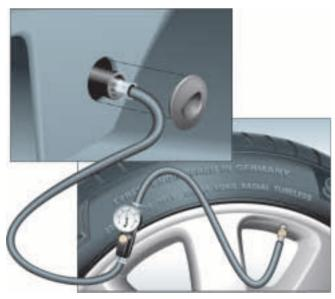
Vehicles with air suspension have a separate tyre inflation connection. This is located under the front right seat. It may only be used to inflate the collapsible spare tyre and tyres filled with puncture sealer.
