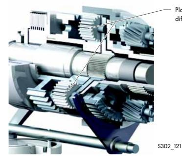
Planetary gear set for centre differential
