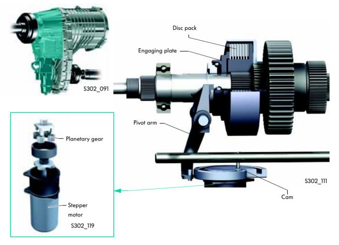
The centre differential lock is a multiple-disc lock that is actuated by an electric motor.
