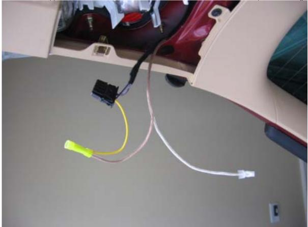
• The P21W bulb can be installed in the bulb holder and snapped back into the tail light housing, don't forget to plug up the connector and snap the access cover back on. The hinge cover can also be re-installed:
