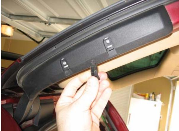
• With the hinge arm cover removed you will be able to access another grommet and use a similar method as before to run the wire through the grommet and down to the access panel where the tail light connector is located:
