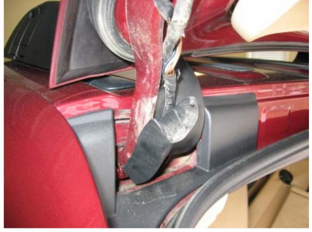
• The headliner clips can be unsnapped on both sides to allow enough room to access one of the rubber grommets where we need to route the wire. Hard to see in this picture, looking up into the cavity on the left you will be able to see the grommets:
