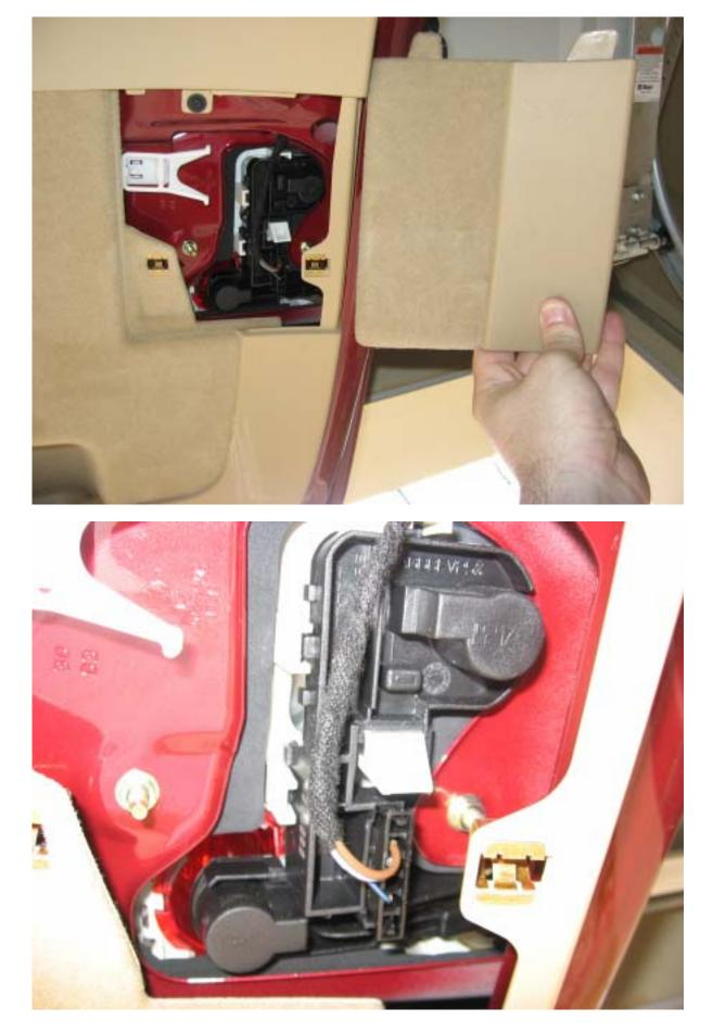
• Pry the connector pin lock up with a screwdriver:
