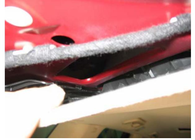
• Your method may vary for this, I have always had good luck using baling wire to both pierce the rubber grommet and to pull the wire through:
