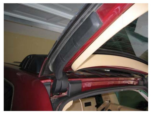
• The wire can now be routed over the headliner and back down to the control module. When running down the pillar I elected to secure the wire to the sunroof drain tube with zip ties. The wire can now be connected to the control module wire installed earlier by using solder or crimp connectors:
