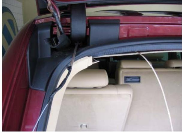
• Once the wire is pulled through that grommet, it will have to be run through the tailgate grommet and to the tail light connector. There is a plastic cover on the hinge arm secured by two Torx screws, the screws are covered by 2 plastic pieces which can be removed by pushing down at the top and sliding down and off:
