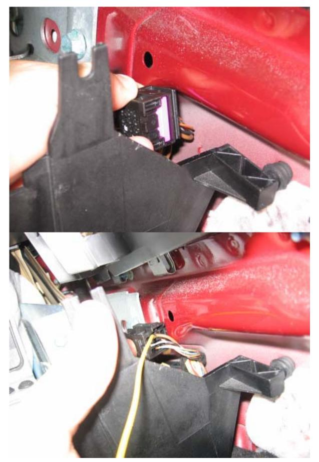
• The remaining pin will be inserted in the tail light plug. Begin by removing the trim panel for the driver's side tail light in the rear door and remove the plug and bulb holder:
