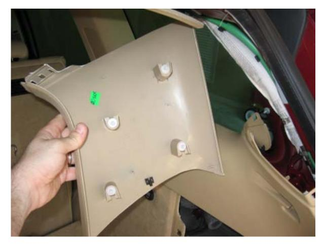
• Now the side panel trim can be removed. The clips seen on the window part of the trim can be reinstalled on the plastic piece prior to reassembly when project is complete:
