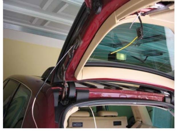
• Once the wire is pulled through it can be connected to the fog light wire installed in the connector earlier with a crimp connector or soldered. I capped off the extra wire I had in case I decide to wire the other side up for a rear fog light later:
