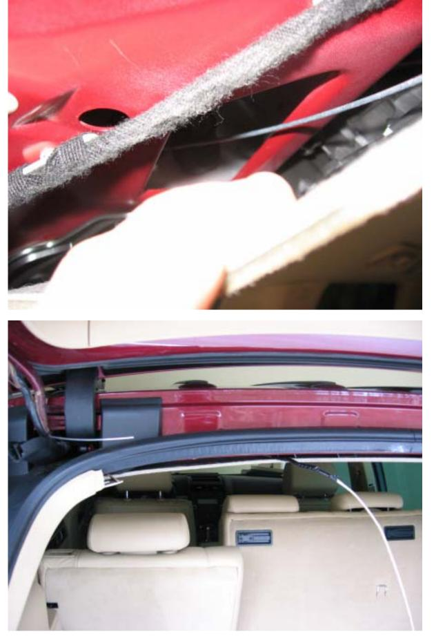
Once I ran the baling wire through to the other side and fished it out the hinge hole, the speaker wire was taped tightly to the baling wire and pulled through. Be careful to route the wire over the looms in the hinge area to keep them off of the piston for the tailgate strut, you can see what I am talking about here by pulling the loom out of the way and using a flashlight to look into the hinge area. It will take a few minutes to get this done (remember, patience is a virtue):
