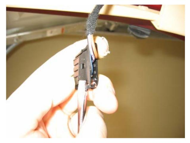
• Insert the pin into socket 2 on the connector (noting the orientation of the other pins) and snap the pin lock down:
