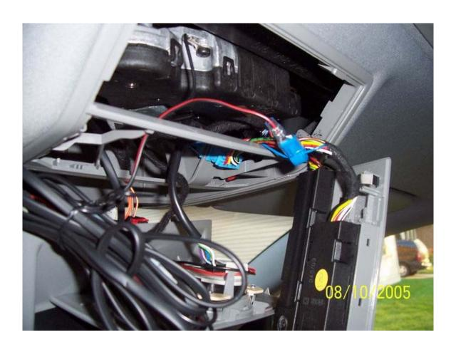
3: Untape the wires going to the HOMELINK module of the overhead console enough that you can access the blue wire (thanks to Spock for determining that this is live switched power). Clamp the scotchlock on the blue wire and attach the power lead of the 8500's hardware kit to the slot created when the scotchlock is installed. Make sure the plastic shielding totally covers the scotchlock as far as possible.
