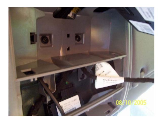
5: Run the wire carefully to the front of the overhead console leaving enough wire to attach the power line to the radar detector wherever you mount it. Replace all of the 4 screws, and all of the lights, and panel covers.
