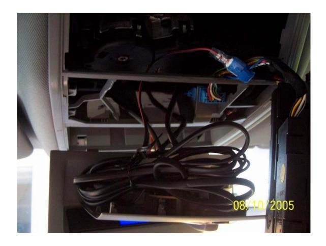
4: Remove the 4 screws that hold the overhead console in place. Watch that the whole thing doesn't fall out! Two are located under the compass panel, and two are located in the homelink antenna panel as shown:
