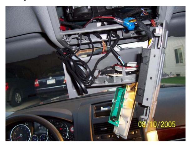
2: Attach the ground wire from the passport install hardwire kit to a ground point inside the overhead console. I used one of the screws on the sunroof control element. You will see it attached in the top of this picture:
