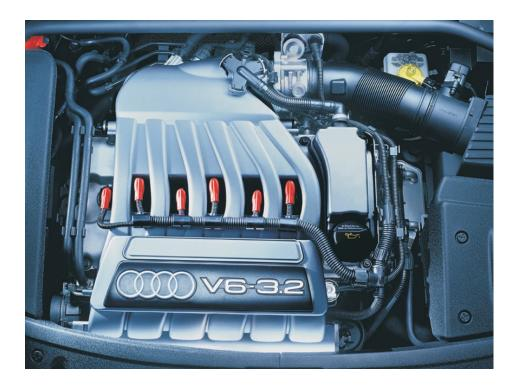
This four-stroke V6 develops an impressive 250 hp at 6300 rpm, and has a broad peak torque range of 236 lb/ft at 2800 to 3200 rpm.
