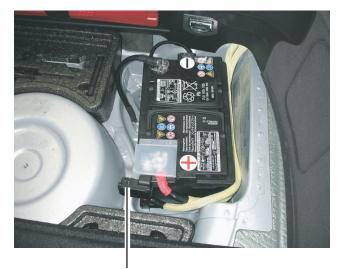
Fuse S138 Connected to Positive Terminal of Battery in Trunk
