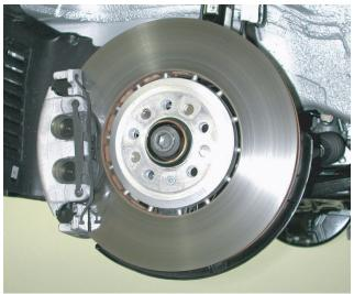
Front Wheel Two-Piece Ventilated Directional Rotors
