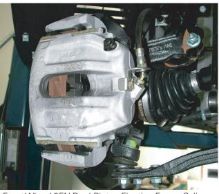
Front Wheel 2FN Dual-Piston Floating Frame Calipers
