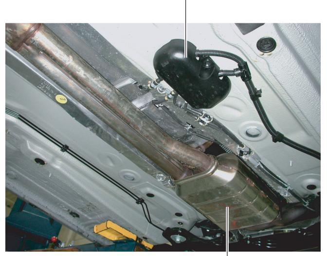
Connector Station for Four Oxygen Sensors
