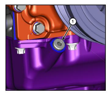
2. Insert the <u>Dipstick 2025600210</u> (1) into the oil level check port until seated squarely on the port opening. Remove the tool and note the oil level (2).
