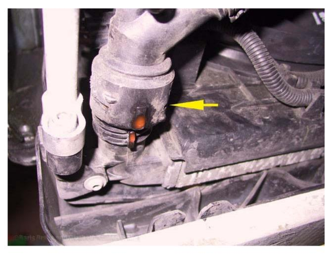
On models with the auxiliary radiator on the passenger side, unclip the return hose leading to the auxiliary radiator.
