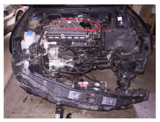
NOTES: Be very careful with how far you move this assembly, as the AC system fittings could be damaged. Also, you can rest the assembly on top of the frame rails when you are not working on the car, and rest the hood on top of this, and it should not come off unless someone yanks on it.
