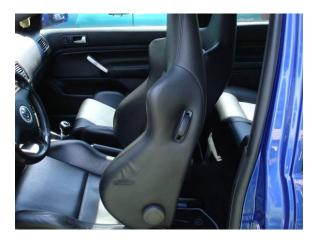
2. If your OEM handle has not pulled out on its own yet, take the OEM handle and pull outward to remove.
