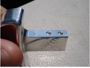
5. Insert new handle to the receiving lever on the seat.
