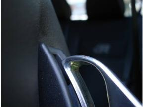
7. Once the handle has been lined up correctly, take the handle and push it down to allow the necessary clearance to tighten the screws with the hex wrench. Be careful not to drop the hex wrench inside the seat when performing this step.
