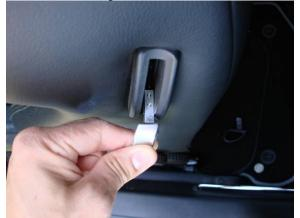
6. Before tightening the handle in place, make sure that it does not rub on the bezel of the seat when moving up and down. You can leave a small gap between the handle and the bezel to prevent any rubbing.
