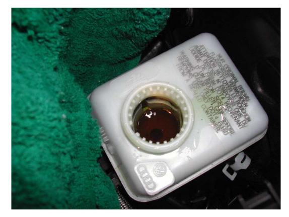
As you can see from that picture, the fluid has some debris floating in it, most likely from the corrosion inhibitors in the factory fluid not working properly (or so I'm told). This upset me as this car is extremely babied, only has 23k miles on it, and I've owned it for 21 months now. This has never happened in any of my other cars.
