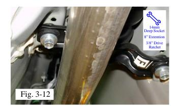
(k) Re-install driveshaft support bearing bracket. (Fig 3-12)
