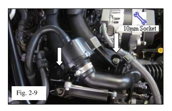
(i) Loosen the two M6 bolts securing the Sound Generator to the intake manifold bracket. (Fig. 2-9)
