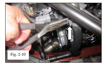
(j) Unclip the Sound Generator tube from the bracket under the passenger strut tower brace. (Fig. 2-10) Fig. 2-11
