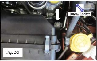
(c) Remove the M6 bolt securing the OEM Air Box to the inner fender. (Fig. 2-3)
