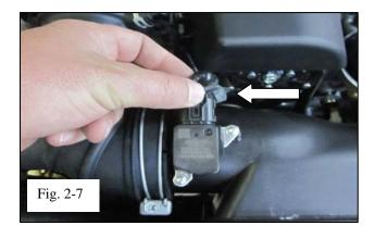
(g) Unplug the MAF sensor and unclip the wiring harness from the OEM Air Box.(Fig. 2-7)
