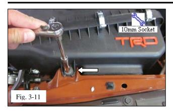
(k) Secure the tab on the TRD Air Box Base to the radiator support with the M6 bolt removed from step 2 (b). (Fig. 3-11)
