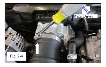
(d) Loosen the hose clamp securing the Air Intake Bellows to the throttle body. (Fig. 2-4)
