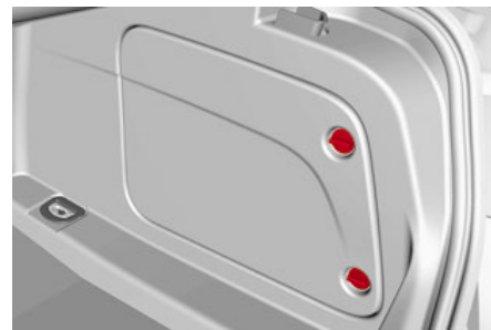
Battery Access Panel
