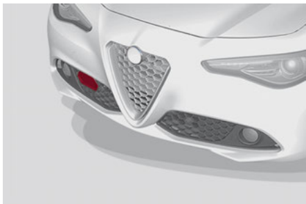
Front Bumper Radar Location
