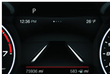
Hand Presence On The Steering Wheel Not Detected Display (Up To 6 Seconds)
