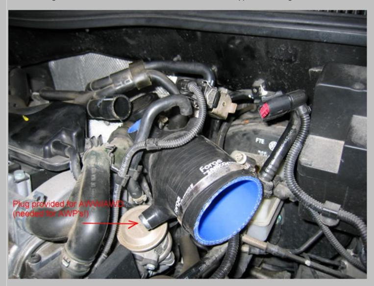
In addition, AWP engine's actually have something that uses the remaining hose outlet on the TIP (see picture). AWD's and AWW's don't need this, so it's plugged up.
