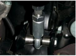
At your earliest opportunity, visit a 8. vehicle alignment shop. Note: You must have a wheel alignment performed before driving more than 250 miles to prevent permanent uneven wear of your tires. After wheel alignment and adjustment of control arms, make sure that the technician aligns ball joint centered on axis with the suspension loaded.
