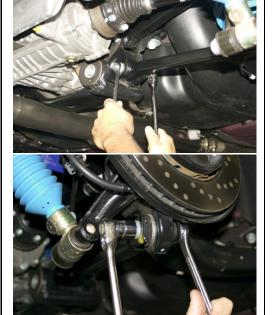
Remove the inner and outer control arm 3. bolts using an 18mm wrench and 18mm socket.
