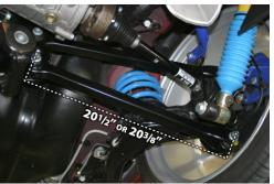
Measure the length of the upper and 2. lower control arms from center of hole to center of hole. The upper arm should measure 203/8", and the lower arm will measure either 203%" or 201/2". If your vehicle is equipped with  $20\frac{1}{2}$ " lower arms, replace the upper arms with The *NEUSPEED* Adjustable these. Control Arms can only be mounted in the lower control arm position. The NEUSPEED Control Arms have been preset at 20%".
