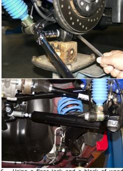
Using a floor jack and a block of wood 6. under cast trailing arm, raise jack to preload the suspension. Torque all control arm bolts to 70Nm (52 ft/lbs). that were either loosened or removed.
