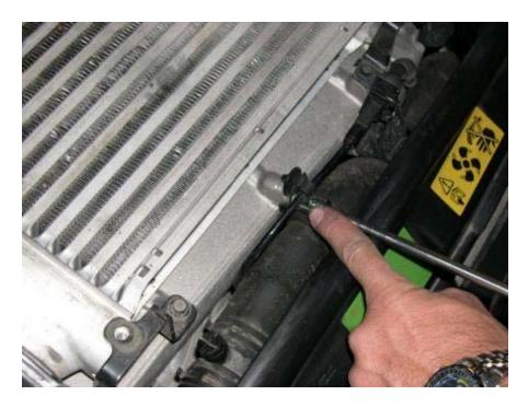
9. Remove the 13mm ground bolt from the passenger side motor mount.
