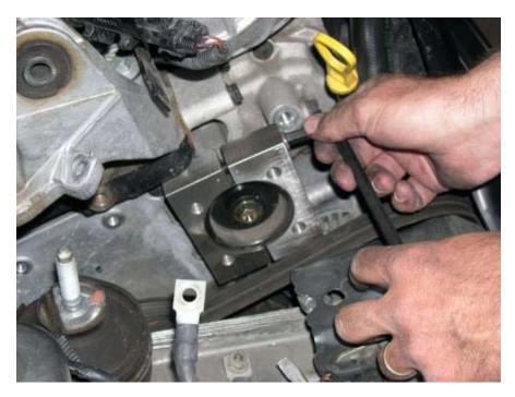
Now install the crow's foot puller onto the removal tool.
