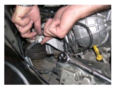
10. I slide the regulator off its bracket to gain more room for the tensioner tool, but you don't really have to. Remove the quick disconnect fittings and use a screwdriver to push the tab on the bracket in slightly and slide it off toward you.
