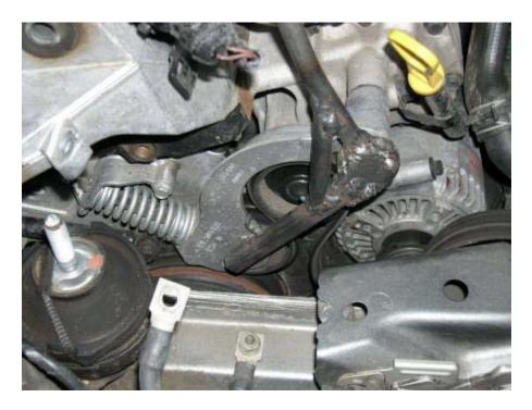
16. Remove the belt tensioner. There are four bolts, two 10mm and two 16mm.
