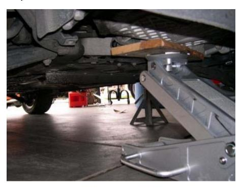
7. Remove the driver side 16mm motor mount bolt. It helps to wiggle as you are pulling it out, and jacking slightly may help as well. It is a little bit of an art, but once you get the hang of it, it is pretty easy (and it is the same thing threading it back in - you get good at it by just wiggling and jacking the motor at the same time).
