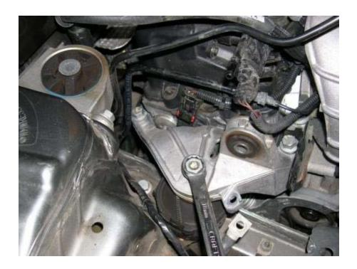
13a. For Model Year 2005-2006, remove the ground strap (#1), then the engine mount nut (#2).
