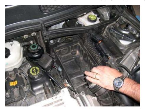
3. Remove the ECU and lower airbox half. Remove the ECU cover (it just has two tabs on each side that squeeze together and pull off), then remove each of the two plugs. These are a little tricky - they have tabs on the end of the plug that pull away from the plug which forces the plug up and off. It's easiest to use a small screwdriver very carefully to pull these tabs away from the plug.
