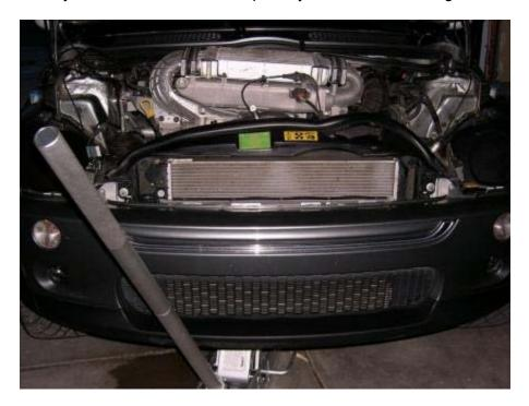
15. Using the belt tensioner tool, remove the tension on the belt and pull the serpentine belt off of the idler gear. The pulley tool is just a big lever with a pin on the end that fits into the two holes in the tensioner itself. The lever fulcrum is the forward 16mm tensioner mounting bolt.
