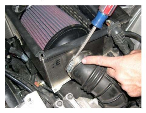
Remove the two #25 torx bolts at the base of the intake heat shield (or if it is the stock box, these same two bolts hold the top of the airbox in place).
