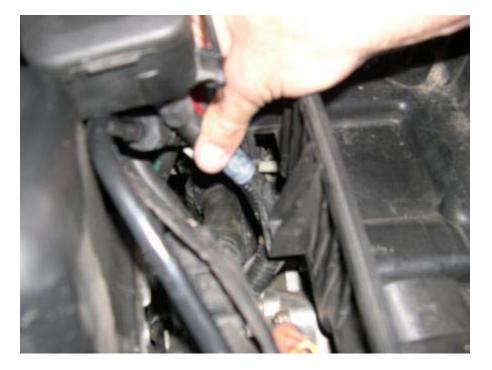
You can now remove the lower airbox half by pulling back and then out.
