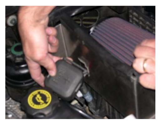
Remove the clamp at the intake boot.
