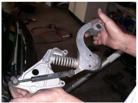
Note the two holes where the tensioner tool is inserted.
