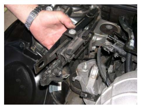
13. Using the 18mm wrench or deep socket, remove the passenger side motor mount nut (MY  $^{\prime}$ 02 -  $^{\prime}$ 04).
