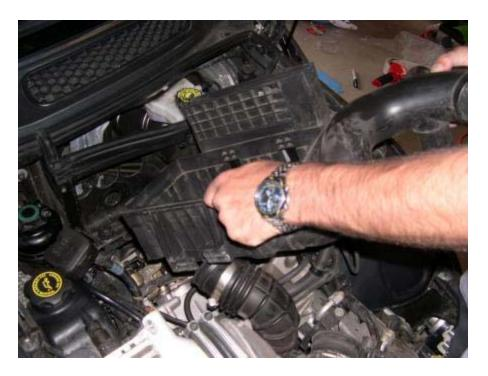
Here's what it looks like with the box removed. Note the two small rubber mounting bolts at the bottom rear of the partition. The box is molded on the underside to fit into these mounts, which is why you had to pull toward the front of the car before you pulled up and out.
