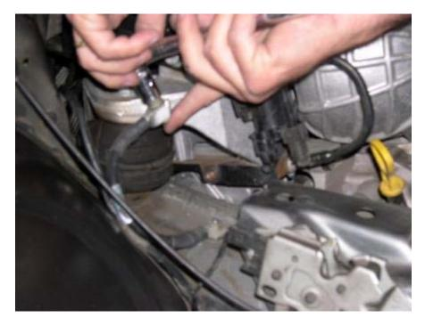
Be careful to hold the bottom of the bolt to prevent it from falling out when you pull the nut off.
