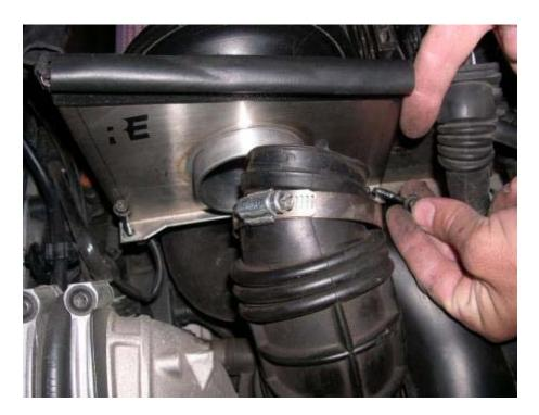
Remove the intake or the panel filter and airbox top (depending on what you have).
