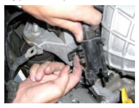
11. There are three hoses attached to the vibration damper bracket. These just pop out of their respective holders (MY '02 - '04). **For Model Year 2005-2006, skip to step 13a**.
