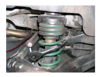
Step 3. Remove one of the rear shock. Start by taking the ABS sensor line and the brake line off of the strut mounts - they just wiggle on and off. Then remove the lower 21mm bolt that holds the strut to the rear hub carrier.
