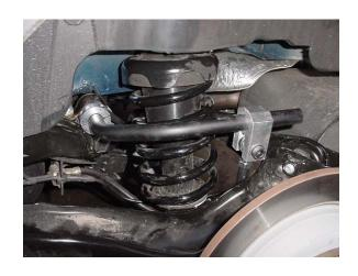
Now double check to make sure that all the nuts and bolts are tightened, then reinstall the wheels.
