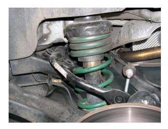
Step 5. Remove the rear subframe mounting 16mm bolts. There are four bolts total, two on each side. Each side has one toward the center of the car, and one toward the outside of the car. The outside bolt is just forward of where the brake line and ABS sensor are mounted to the rear subframe. Once you get under the car, they become much more obvious. The inner bolt is shorter than the outer bolt. This is the inner bolt location:
