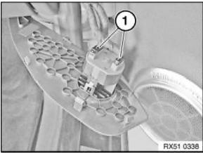
With passenger airbag deactivation optional extra only: Unlock plug connections (1) and disconnect.
