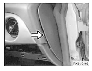
Lever out cover on left and right in direction of arrow.
