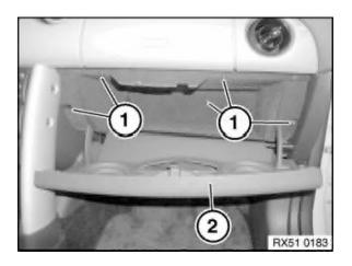
Release screws (1). Remove glovebox (2).
