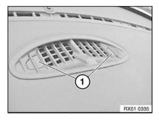
Lever out cover caps (1) in ventilation grille and release screws underneath.
