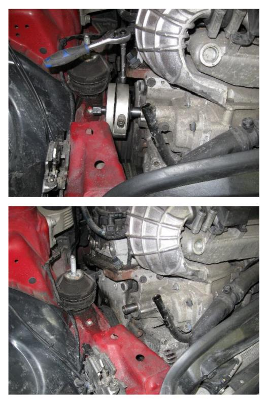
9. Mount the inside piece of the KMT pulley. If it is very tight you can use some sandpaper (1200) on the inside. Put it as back as you can on the shaft. Take the outside piece of the pulley and 4 bolts. Use loctite on them. Hold the outside piece of the pulley to the shaft and screw down the bolts. Tight them as much as you can hold the pulley.
