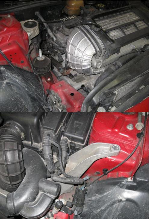
http://www.kavsmotorsport.com Mini Cooper S tuning - smaller pulley for the Mini Cooper S 5. Remove the 6mm screw which holds the radiator hose at the front (a little lower than the intercooler).
