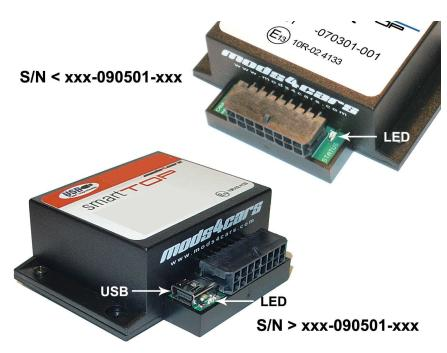
The green InstallAID™ LED signals a correct installation and shows the status of the module.
