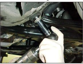
c) Using the same 16mm socket and a long extension, remove the two bolts (1 per side) as the sub-frame turns up and just forward of the axle line.
