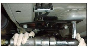
b) Using the same 16mm socket, remove the 2 bolts (1 per side) located at the rear-inboard edge of each wheel well.
