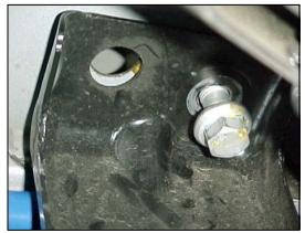
7/ The sub-frame should be loose. Apply pressure to the sub-frame so that the bar (without the brackets and bushings) can be pulled out from one side.
