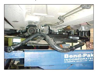
9/ **Before installing the bushings or brackets**, install the HSport bar the same way in which you removed the stock bar. The center HSport sticker faces righ-side up and to the rear of the vehicle.
