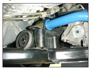
Now, start with the bushing bracket bolts, then the steering rack torx bolts and reinstall all the rest of the sub-frame hardware. **Make sure ALL bolts are reinstalled and that they are tight and secure!**
