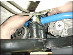
13/ Finally, make sure that the end-link nuts are secure by using the 5mm allen with the wrench. We recommend that you start in the 'soft' position which is the hole towards the bar end.
