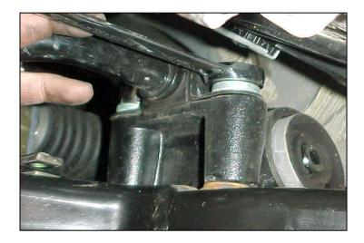
8/ Finally, the bar is free and you are ready to remove it. Do this by simply rotating the center to lift the ends over the steering arms, then pull straight out towards the rear of the vehicle. You may have to maneuver the bar to better position it as it comes out but be patient.
