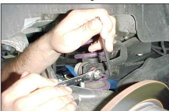
4/ Next, remove the two-spring/shock assemblies (only one side is required but both removed makes the job easier) using a 13mm socket with extension for the two upper bolts and a 21mm socket for the lower bolt as shown.
