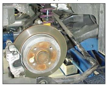
Once the stock bar is out, slide the Hotchkis bar in without the bushings and brackets attached. Once the bar is in the approximate stock location, use the remaining grease on the inside of the rear bushings and slip them over the bar. Then install the supplied bushing brackets with the grease fittings pointing to the outside.
