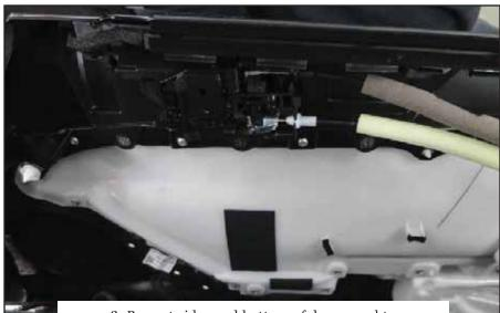
3. Pry out sides and bottom of door panel to release eight (8) clips, disconnect harnesses and door lock/release assembly, then remove door panel.
