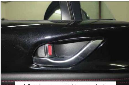
1. Pry out screw cover behind door release handle and remove one (1) exposed Phillips screw.
