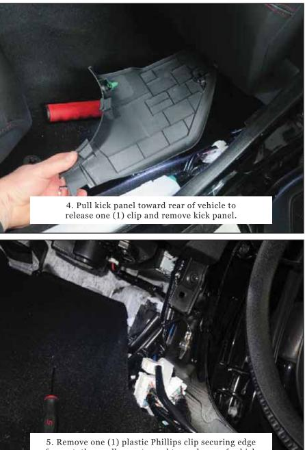
5. Remove one (1) plastic Phillips clip securing edge of carpet, then pull carpet panel toward rear of vehicle.
