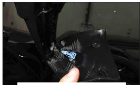
Starting at top edge, pry off front pillar trim panel to release two (2) clips, disconnect harness and remove trim panel.
