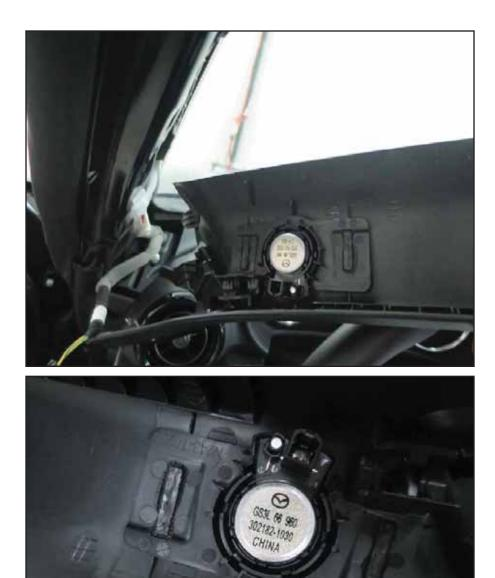
2. Pry tweeter off pillar trim panel to release clips and remove tweeter.
