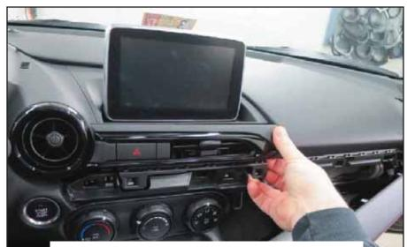
2. Pry out center dash vent/hazard switch panel to release seven (7) clips, disconnect harness and remove panel.
