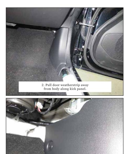
3. Remove one (1) center pushpin clip from the passenger's side kick panel by first prying out center pin, then prying out entire clip.
