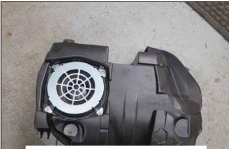
8. Remove four (4) Phillips screws securing subwoofer to enclosure, disconnect harness and remove subwoofer.
