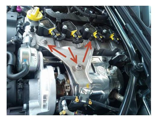
4. Remove the three 10mm bolts shown below. Use a 10mm wrench for the lower bolt. Once removed, you can lift the heat shield and set it aside.
