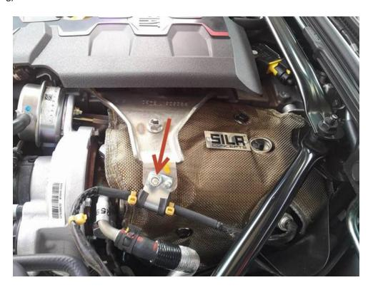
12. Peel off the protective cover on the SILA Concepts plate.
