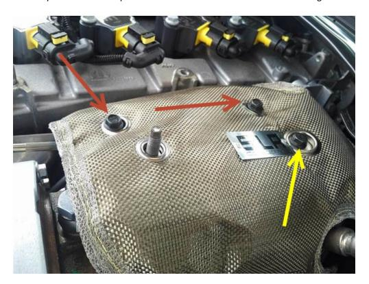
9. Using the third bolt provided with the Thermal Blanket or one of the bolts from step 4, loosely tighten the bolt at the side, then tighten all four bolts to approximately **25-30 in/lb** (hand snug).
