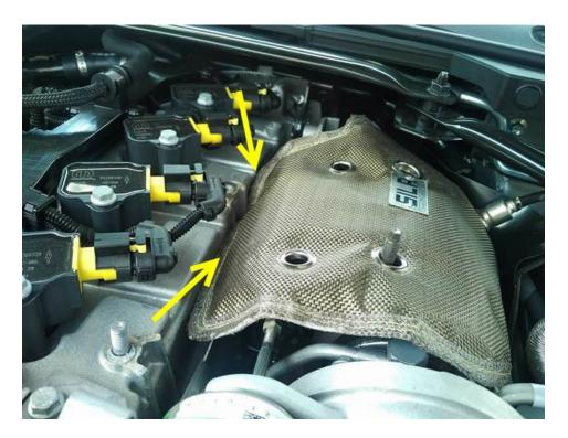
8. Using the bolts that came with your Thermal Blanket, loosely tighten the two upper bolts. Use one of the bolts you took off in step 4 where indicated below toward the bottom right.
