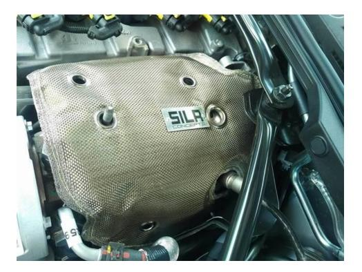
7. Tuck the Thermal Blanket over the side of the heat shield bracket.
