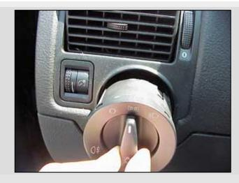
Remove the headlight switch by pushing in and turning clockwise on the switch. The switch will now pull straight out from the dashboard.
