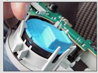
Remove the old sunroof switch from the old panel. Pry back on each of the retaining clips. Work the switch out slowly.
