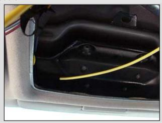
Run the long wire from the ECS thru the headliner, thru to the windshield or straight over to the A-pillar. You will need to run this wire down to the back of the headlight switch.
