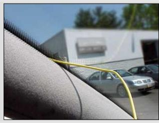
Continue to run the wire down the A-pillar to the headlight switch. You can use a credit card or simillar to tuck the wire between the glass and cover, this actually works very well. (The A-Pillar cover can be removed to better hide this wire.)
