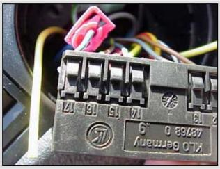
Locate pin 17 on the harness connecting to the light switch. Using the supplied Scotch-Lock, tap into the the GRAY wire with BLUE stripe coming from the #17 location. Re-Install the headlight, wait till dark, turn on the lights and feel the love.
