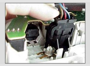
Disconnect harness from light panel. Use a screw driver to free each side of the plug.
