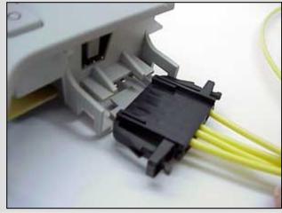
Install each end of the ECS wiring harness into the existing car harness and the new W8 overhead light module.
