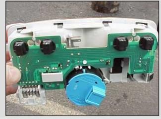
Install the old knob into the new W8 light panel. Note the orintation of the black/blue/black tab on the switch; It should face the bulb sockets in the panel. Before seating the switch, flip the panel over and check that the knob rotates correctly withing the markings on the panel.
