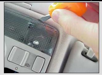
Using a flat bladed screw driver or pick, pull down on the leading edge of the lens cover.
