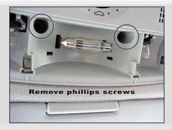
Remove the two phillips screws from behind the lens cover.
