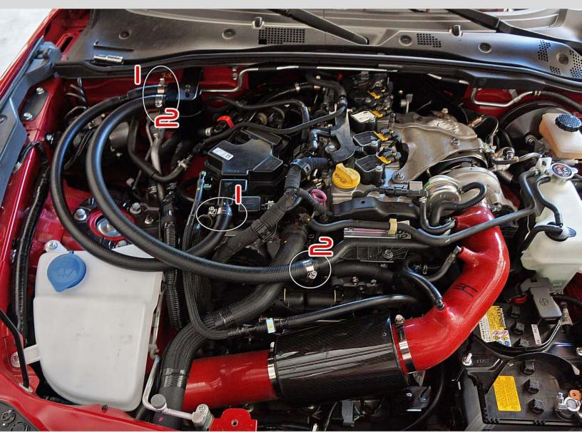
There are two joined connection points as shown above. **Hose clamps are 8mm hex.** All clamps must be tight but please do not over tighten.
