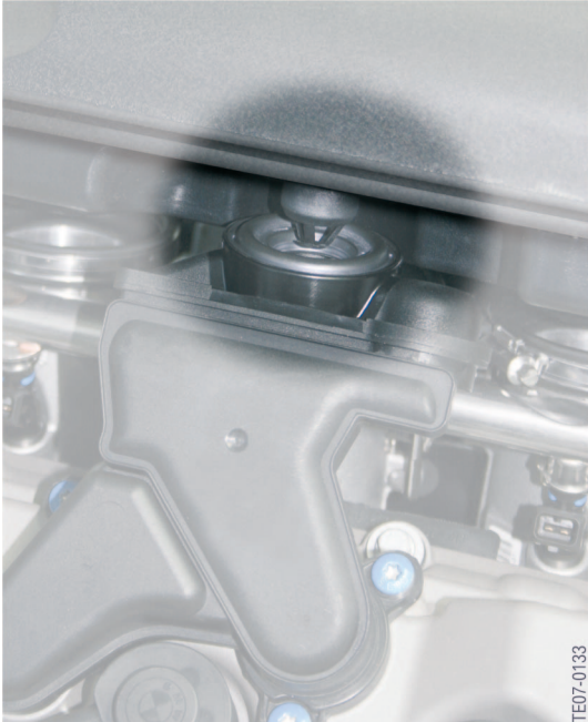
47 - S65B40 Oil separator connection point to the intake manifold
