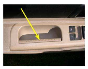
3. Insert a screwdriver or other strong, thin tool into the crack between the inner and outer pieces, as shown below, and carefully spread them apart. Be careful not to harm the soft-touch coating on the handle pieces - you may want to protect the tool with a thin rag. Although a screwdriver is shown in the picture, I actually prefer a tool with a wider blade, such as a putty or spackling knife - it has always been easier for me to get the handles off with one of these.
