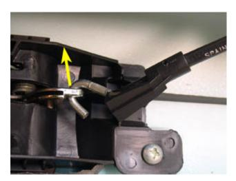
22. The picture below is a side view of the cable retaining clip to help illustrate how to detach it. You need to pull outwards on the front of the clip (1) to clear the tabs and then slide it to the rear (2).
