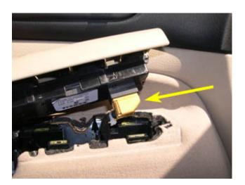
7. If your main door and window controls unit is not working properly (like mine), you can replace it by removing the three medium Phillips screws (yellow arrow in picture below) that attach it to the main handle piece. If your unit is working properly and/or you do not want to replace it, ignore this step.
