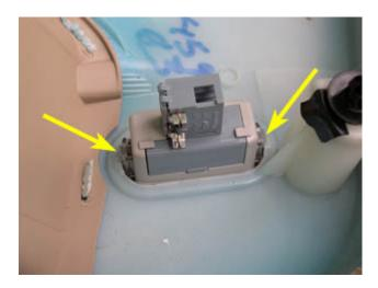
32. To view your window regulator clips, remove the two rubber plugs (one shown in picture below) with a screwdriver and raise the window until you can see the clips at the bottom of the window glass through the holes (this will require you to temporarily reconnect the main driver's window and door lock controls).
