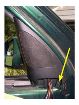
27. Pull the speaker grille off of the door. The inside of the grille is also attached to the door by three tabs which are indicated by the arrows in the picture below.
