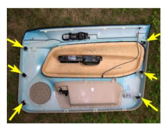
18. Starting with the top, rear corner, pull the door panel up and out of the window seal, as shown below.
