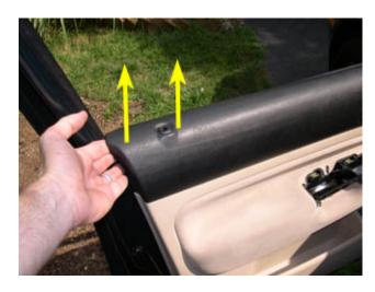
19. Do the same with the top, front corner of the door panel, as shown below. The door panel should now be disconnected from the door except for the electrical and door lock cable connections in between the panel and the door. You can rest the door panel back into the window seal if you want to take a break or reach for a tool.
