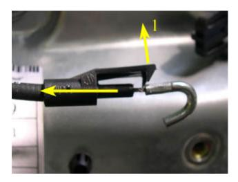
23. After the lock cable is disconnected from the unlock handle, unclip the electrical connections for the front driver's door (mirror switch, alarm LED, door light, trunk release, gas door release and the speakers) or the front passenger's door (door locks, door light and speakers). You should now be able to remove the door panel from the car.
