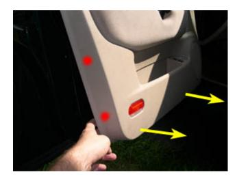
17. The picture below of the inside of the door panel shows the location of the six snaps. (This picture is for reference only and was taken later in the DIY. The door panel should not be off yet).
