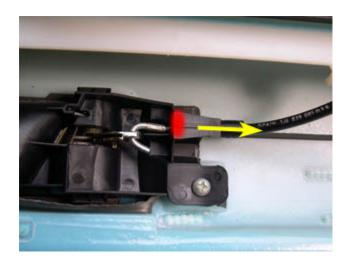
21. Once the clip is unhooked, remove the cable from the groove in the unlock handle assembly and then detach the hook from the unlock handle, as shown below.
