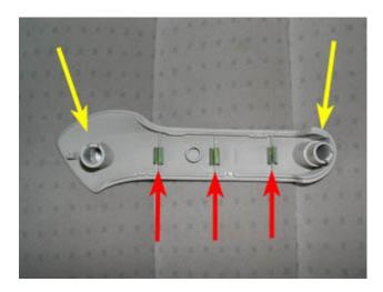
13. The picture below shows the inner handle piece still attached to the door panel. The handle piece is attached to the door panel with three medium Phillips screws (red arrows) and the door panel is secured to the door with 2 large Phillips screws (yellow arrows). If you want to remove the inner handle piece from the door panel, remove all five screws. If you are just taking the door panel off, only remove the two large screws indicated by the yellow arrows.
