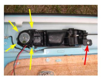
25. Once the front edge of the handle assembly is pushed out (1), slide the assembly toward the front of the car to remove (2).
