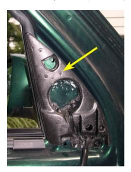
29. The sideview mirror assembly is attached to the door with a single T45 Torx screw (thanks bluetoyota for the size). Remove this screw and pull the mirror assembly off of the door - be careful not to harm the wires for the mirror glass heater element and the mirror motor.
