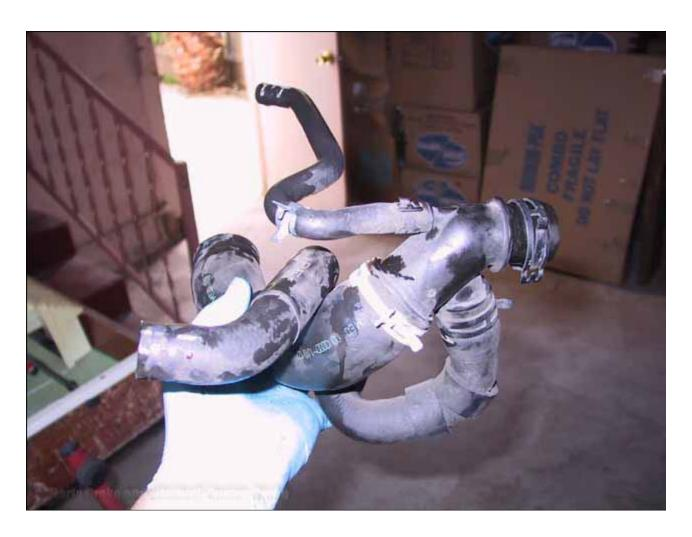
5: Now remove the lower thermostat housing hose. This one is particularly difficult to get at as well. See the yellow arrow in this image:
