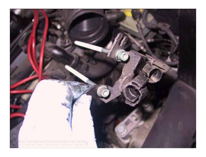
Here is a picture of where this smaller one is located. Be sure you have the right bolt, as the other two pictured are for the timing chain cover.
