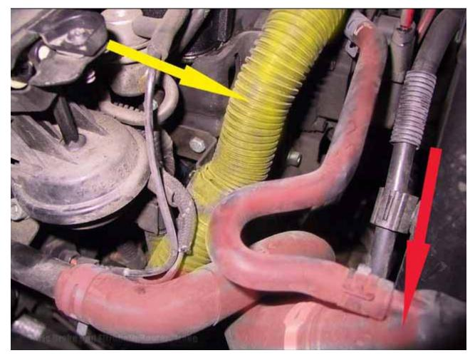
3: Get the smog pump supply line out. This is the plastic corrugated hose that has the rubber protectors on it that seems to be snaking around the outside of this morass. You may have to cut a zip tie. Squeeze the connectors on the fatter textured sides and pull straight back to get them off. The connectors may stick, keep in mind that they are sealed with o-rings so see if a little twist sets them free.
