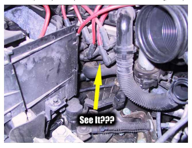
2: Remove the top engine cover (the thing with the chrome Vr6 emblem). This gives you easier access to the coolant and smog pump lines just beneath the coil. To do this first pull the spark plug wires using the tool and pull them from their channels, then remove the six or so T25 Torx screws. Then remove the oil filler cap and pull the cover, and replace the oil filler cap. I would also put the screws for the cover back in their holes just to keep track of them.
