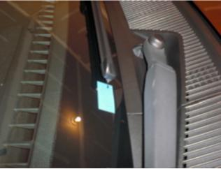
3. Remove the two rubber caps on the windshield wiper arms. These just pull straight off. Driver side removal is shown below. Repeat for the passenger side windshield wiper.
