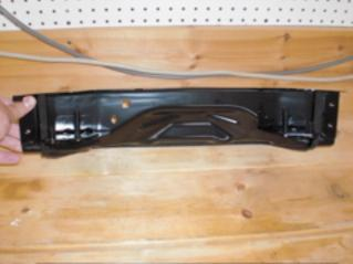
Pictured below is a comparison of the cowl panel with and without the FSTB mounts (left). The only difference between the cowl panel with the FSTB mounts is the welded mounting brackets with the mounting bolts (right):
