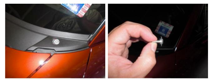
8. Open the hood. Detach the rubber weatherstrip on the engine compartment side of the plastic cowl. There are several plastic push clips holding this seal and the plastic wiper cowl to the metal lip. You only need to remove the clips that go through both the plastic and the metal lip. Squeeze the clips from the bottom to pull them out. The weatherstrip can remain attached to the cowl.
