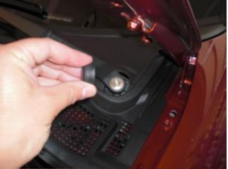
4. Remove the nuts (14 mm) holding the windshield wipers on. Passenger side removal is shown below. Repeat for the driver side windshield wiper.
