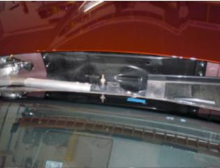
11. Unbolt the two 10 mm bolts that hold the windshield wiper motor. Note: this is not necessary to remove the original cowl panel, but the extra clearance will be needed to install the new cowl panel (with the FSTB brackets).
