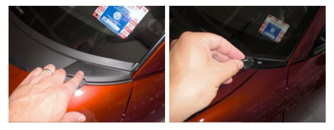
7. Remove the screw (Phillips head) under each plastic cap.
