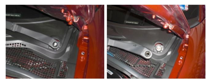
6. Remove the plastic caps on each side of the plastic cowl panel. Use a thin knife to **gently** pry up on the cap. Driver's side is shown; repeat for passenger side.
