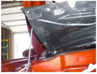
10. Remove the plastic cowl piece by sliding it toward the front of the car about an inch and gently pulling up on it. Pull the cover out toward the rear of the car. The plastic cowl is actually two pieces but should be removed as a single unit (the weatherstrip and wiper fluid hose is still attached to both sides).
