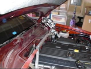
20. Place the new cowl panel in place by sliding it in at an angle while maneuvering the air conditioning lines over the long bolts that are welded to the cowl panel bracket. Bolt the new cowl panel into place with the 8 bolts that held in the original cowl panel.
