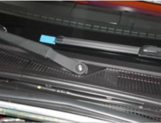
5. **Gently** wiggle the arms loose. It may be helpful to lift the wiper arms up off the windshield to pull the arms off the mounts (if doing this be careful when opening and closing the hood so the wiper arms are not crushed).
