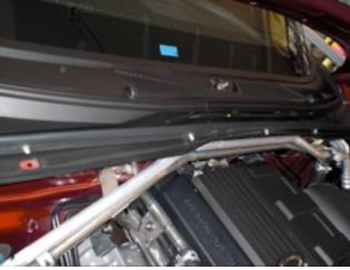
9. Lift up on the plastic cowl. Detach the plastic washer fluid hose at the plastic Y-connector underneath the plastic cowl (left). Unhook the hose from the hooks on the underside of the plastic cowl and pull the hose out of the hole on the passenger side of the plastic cowl.
