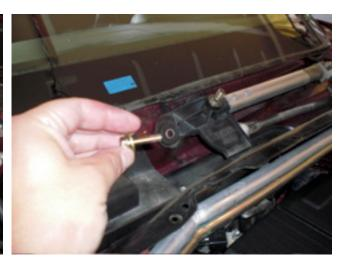
12. Remove the plastic panel on the passenger side next to the wiper motor by unscrewing the five plastic screw clips.
