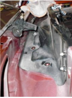
15. Two bolts have been removed per the left picture below and the final two bolts have been removed per the right picture below. There is not a lot or room to work here so you may have to be creative with the tools (and patient) to get everything unbolted. Be careful not to drop any of the bolts/nuts!
