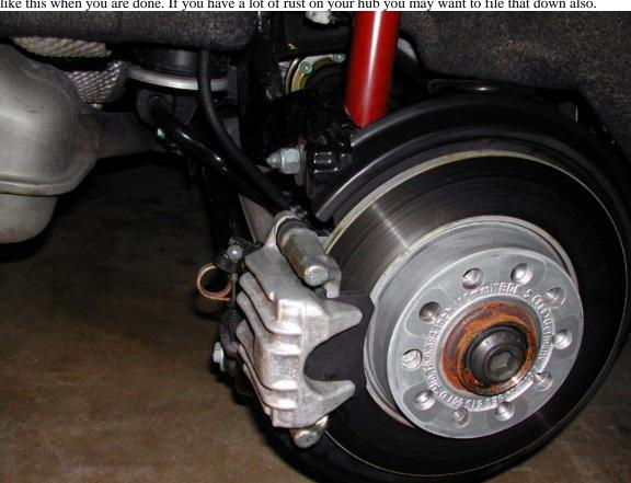
10. Re-attach wheel. Be sure to use the star pattern, and if you have a safety bolt be sure to put that one directly opposite of the valve stem. Also tighten that one last. Torque to 92 lbs/ft.
