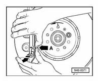
Press rotaining spring so far in direction of (arrow -\Lambda-) until it can be pressed out of the bore of the brake caliper.
