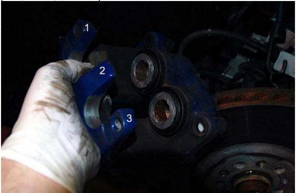
Pop the wear sensor into the new pad, snap the pad into the two pistons, put the front pad in the mounting bracket, and screw back in the caliper screws and put back the front retaining clip – you're all set! I did not have to push back the pistons as I only have 4900 miles and the pads weren't very worn. If you did have to push back the pistons, I would just stick a big set of pliers in-between the pads and expand them, thus pushing back the pistons.
