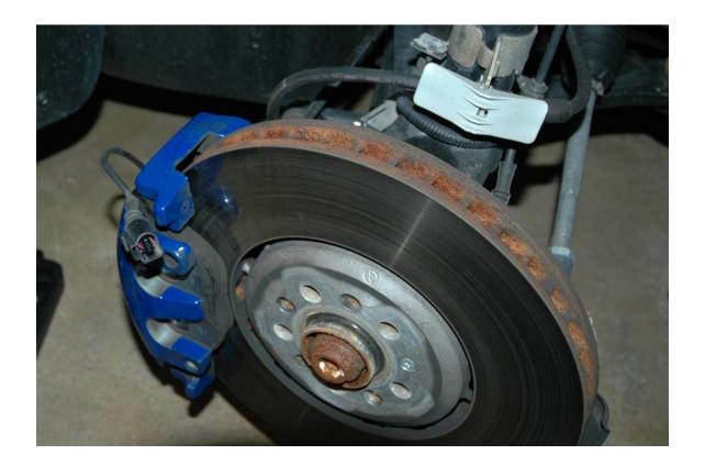
Now you just have to remove the bottom caliper bolt and the caliper will slide off. Now remove the back pad and carefully remove the wear sensor as follows:
