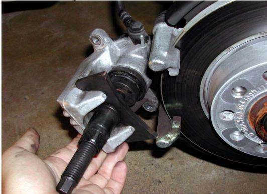
You will hand tighten it until it is locked in there, then get a 14mm socket and tighten so it will turn and push in on the piston. If your old pads were fairly new (mind only have 4k miles) then you won't need to compress the piston very much.
