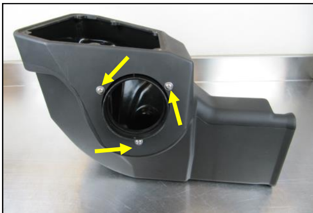
7. Install the Filter Adapter onto the Cold Air Box as shown, using the three 1/4-20 Button Head Screws and 1/4" Flat Washers
