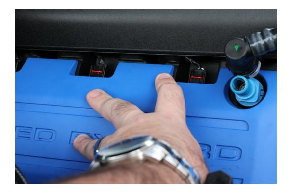
6. Replace the Oil Cap, and snap the PCV Tube into the receiver.
