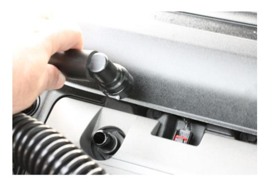
8. Remove the stock Coil Cover by gently unsnapping it from the mounting points.
