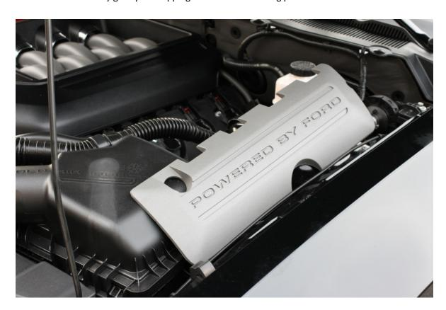
9. Slide the correct Boss 302 Coil Cover into position, and press firmly to lock it into place – replace the PCV Tube.
