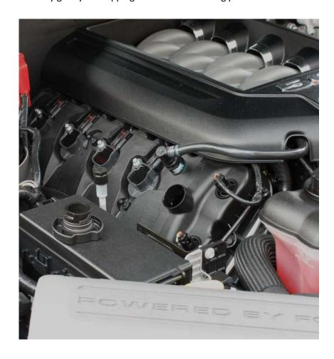
5. Slide the correct Boss 302 Coil Cover into position, and press firmly to snap it into place.
