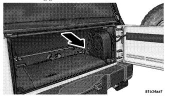
• Unzip the rear window starting at the right lower corner of the window. Pull the zipper up, across the top and down to the left lower corner. **Zipper pulls will stay on the rear window.** Pull down on the rear window to disengage it from the zipper on the top cover.
