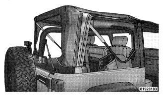
9. Partially install the sail panel retainers into the body side channel, leaving the last 3 in (7.6 cm) toward the rear window loose (on both sides). Pulling down on the rear roof bow (3–bow) will aid to reach the channel with the retainers.
