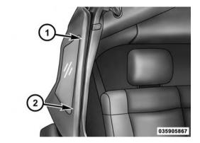
1 — Incorrect Insertion 2 — Correct Insertion
