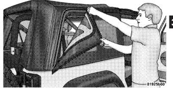
10. Once unzipped, remove the side window retainers from the door channel and body side channel. Repeat this step on the opposite side.
