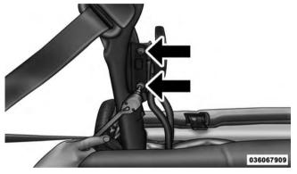
6. Lift the soft top in an upward motion to release the pivot bracket from the sport bar bracket mounting tab.
