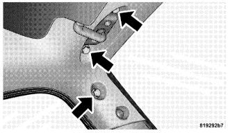
5. Install the lower windshield plates with the six black round-headed Torx<sup>®</sup> head screws (using a #40 Torx<sup>®</sup> head driver) on each side of the base of the windshield.
