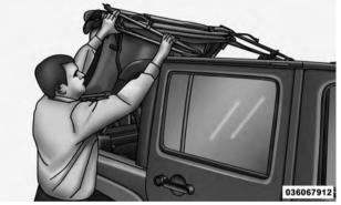
6. Ensure that the top locks into the Sunrider<sup>®</sup> locking mechanisms that are located above the front of the rear doors.
