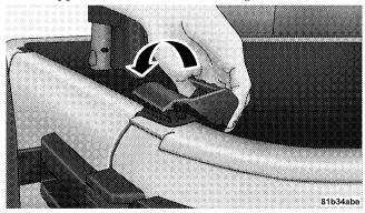
8. Move to the rear of the vehicle and gently pull the sail panels over the rear roof bow.
