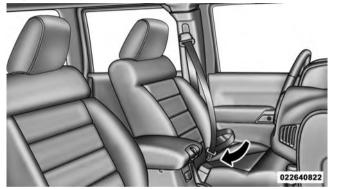
Inserting Latch Plate Into Buckle
