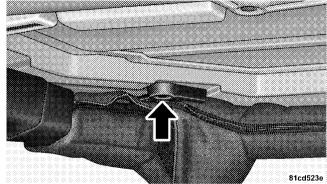
5. Unlatch the header panel latch located at the top of the windshield.
