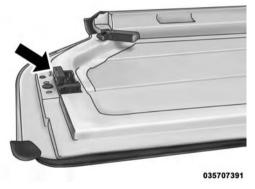
**NOTE:** The front panel(s) must be positioned properly to ensure sealing. Set the panels on the windshield frame so that there is no overhang. Also, make sure that the panels are sitting flush with the body.
