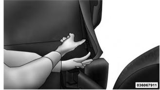
3. Release header latches from the windshield frame.
