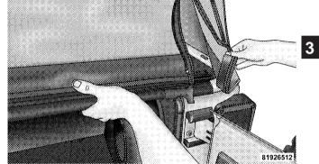
17. Insert the rear window retainer into the swing gate bracket on both the left and right sides.
