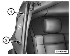
8. Insert the retainer along the bottom edge of the window into the bottom side channel, beginning at the front and working to the rear of the vehicle. Finish by closing the zipper completely and attaching the Velcro<sup>®</sup> along the top and rear of the window. Repeat this step for the opposite side.
