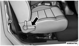
With the seat forward, pull the entire seat assembly toward the instrument panel.
