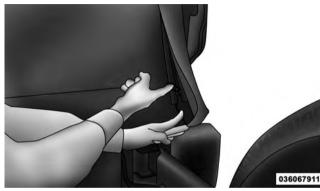
3. Release header latches from the windshield frame.
