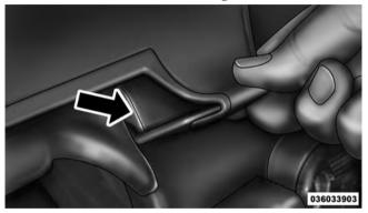
19. Close the header latches and return the sun visors to their secured position.
