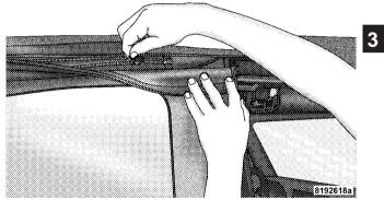
11. Insert the front retainer of the window into the door channel, making sure the retainer is fully seated and properly positioned on the door frame. Failure to do so can result in wind and water leaks or damage to the window.
