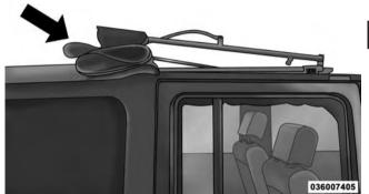
6. Secure the top by using the two provided straps. Each strap will wrap around the side bow and Velcro<sup>®</sup> to itself; use one strap on each side of the vehicle.
