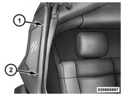
7. Insert the retainer along the bottom edge of the window into the bottom side channel, beginning at the front and working to the rear of the vehicle. Finish by closing the zipper completely and attaching the Velcro<sup>®</sup> along the top and rear of the window. Repeat this step for the opposite side.
