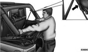
5. Screw the pivot screws back into place using a #T30 Torx<sup>®</sup> head driver. Secure them until they are snug, being careful not to cross-thread the screws or overtighten.
