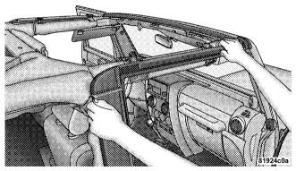
4. Screw the knobs back into the door frame and fold for storage. Store in a secure location.
