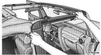
5. Starting with the front knob, screw in and tighten both **Door Frame Installation — Four-Door Models** knobs. Repeat on the other side.
