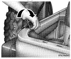
14. Completely release the latches from the loops on the windshield frame. If your vehicle is not equipped with the Sunrider<sup>®</sup> package, proceed to Step 15.
