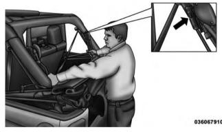
7. Reinstall the hard top. Refer to "Freedom Top Three-Piece Modular Hard Top — Front/Rear Panel Installation" in this section.
