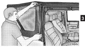
6. Insert the front retainer of the window into the door channel, making sure the retainer is fully seated and properly positioned on the door frame. Failure to do so can result in wind and water leaks or damage to the window.
