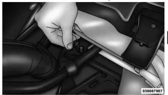
4. Slide the tether strap up the side bow and attach to pivot bracket to secure side bows before removing soft top (both sides).
