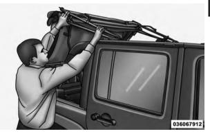
Gently slide the side bows off the door frame track and lower the top down into the vehicle.
