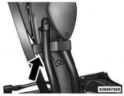
5. Remove the soft top bow assembly pivot bracket screws (two per side) from the sport bar using a #T30 Torx<sup>®</sup> head driver.
